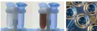
Fig.4: Magnetic Separation. Estapor Magnetic Microspheres are compatible with any automated platform using 96-Well plate (right) or manual system using simple tubes (left).
