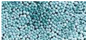
Fig. 2: TEM view of Estapor® SuperParamagnetic Microspheres, reference M1-070/40
