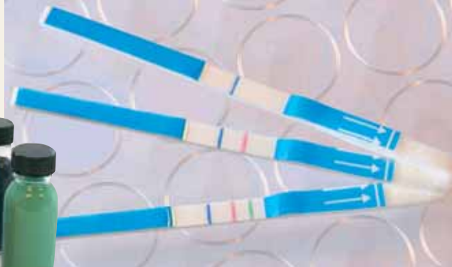
Fig. 2: Lateral Flow Tests using Estapor Dyed Microspheres (reference: K1-030 blue for the control and K1-030 red for the sample).
